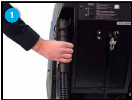
Recovery tank drain hose
