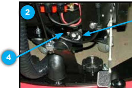
2 Solution flow adjustment knob and wire connections
