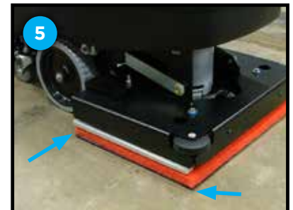
Proper alignment of pad
