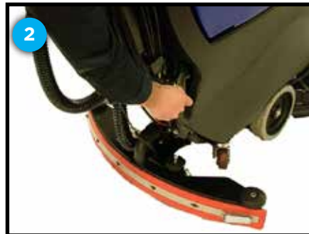
Locking in high down pressure setting by lifting foot lever
