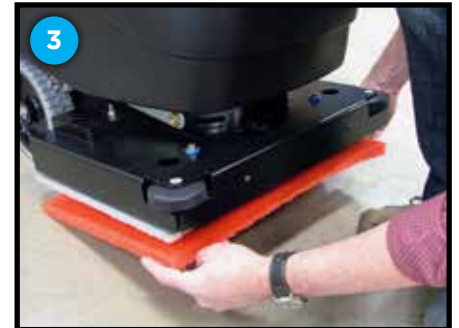
3 For pad removal on the orbital unit, simply pull off the pad
