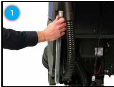
1 Check sight gage hose for solution level
