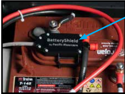
BatteryShield optical sensor on Trojan battery
