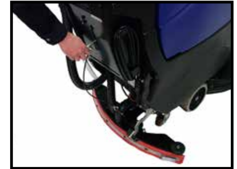
Lowering the squeegee assembly
