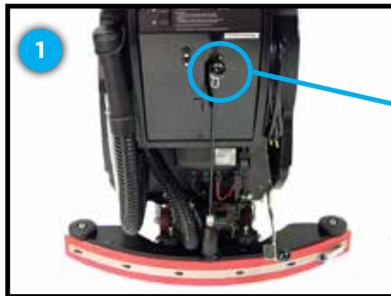
Squeegee assembly in transport/storage position
