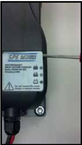
Use small screw driver to lift label off charger
