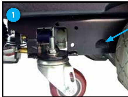
Tie down location on main frame
