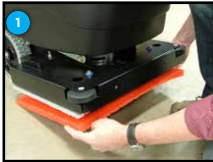
Align the front corners of the pad and press to adhere
