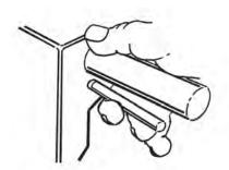
\*when you start the machine with the pad lifted off the floor. Once it starts spinning then you may lower to the floor and start working.
