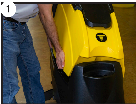
To access battery compartment, tilt recovery tank to fully open position
