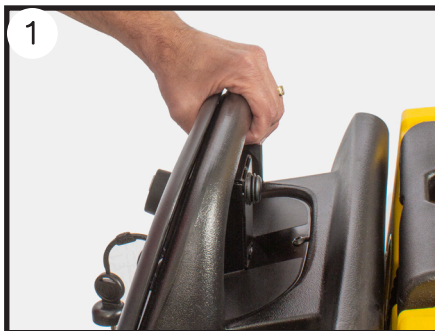
Activating the handle trigger
