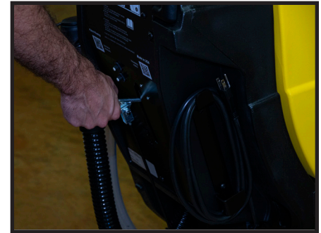
Lowering the squeegee assembly
