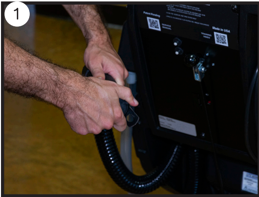
Check for clog in the restriction collar
