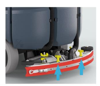
**5.** Check the squeegee blades are not damaged and install the squeegee by turning the yellow knobs. Check the height of the squeegee by adjusting the castor wheels and the angle knob.
