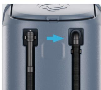
**4.** Verify that the suction hose is firmly connected to the recovery tank inlet.
