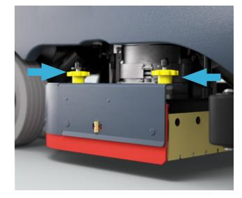
**6.** Install the brushes by removing the side blades. The side blades are removed by unscrewing the fasteners.
