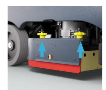
1. Remove side skirt assembly and verify brush installation and condition.
