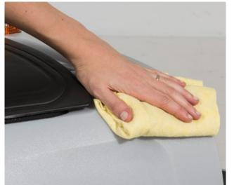
18. Clean the machine using a damp cloth and where needed use a neutral cleaning product.
