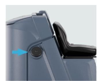
3. Fill the tank with clean water. The clean water temperature must not exceed 40 °C (104F).
