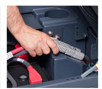
3. Check battery cables are well connected together.
