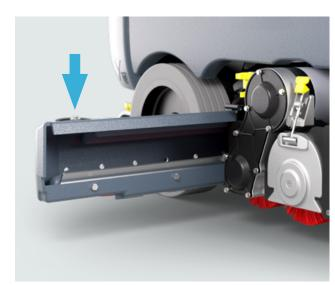
14. Slide out, check, empty and clean the debris hopper (cylindrical version).
