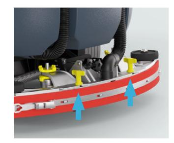
**16.** Untighten the yellow knobs, take **17.** Clean the filter: the squeegee off and remove debris. Check and clean the squeegee blades.
