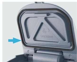
4. Recovery tank seal cover must be correctly installed and in good condition to maintain good suction performance at the squeegee.
