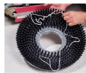
**15.** Turn the brushes counter clock wise and remove the brushes or pad holders. Rinse the brushes or pads in warm water and hang up to dry.
