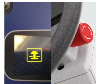
2. E-stop icon appears on display when E-stop switch is engaged. Twist E-stop switch until it pops out to enable machine function.
