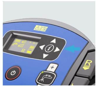
2. Press "I" scroll down to faults and 3. Turn brushes counter clockwise press ">" button to view faults.
