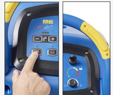
7. Press the OneTouch™ scrub button to enable scrubbing. The vacuum will start. Push on one of the two switches 1/2 second to install the brush. Brush will automatically install.
