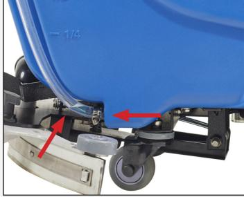
2. Daily: Empty the clean water tank using the solution tank drain hose and sight tube.
