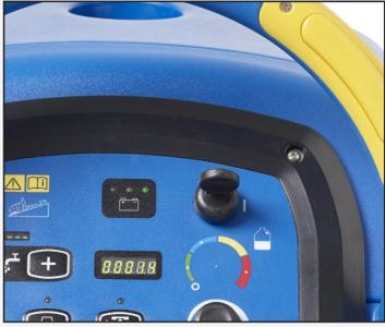
1. Turn on the key and verify there is enough battery power to complete the work. Charge batteries as required.
