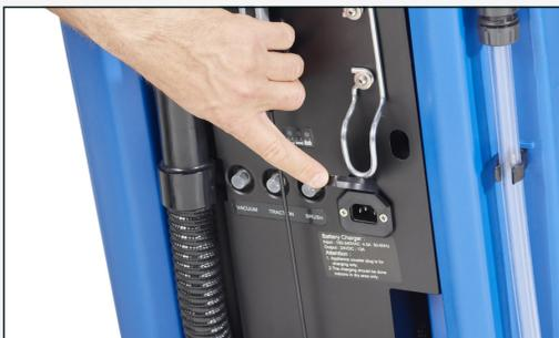
8. Daily: Charge the machine when not in use using the supplied AC cord and on-board charger receptacle.
