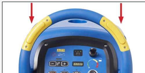
9. Press left, right or both yellow palm switches to move the machine forward.
