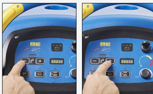
12. Press the + or - solution buttons to increase or decrease the water flow rate and to turn water off.
