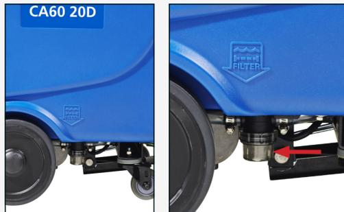
6. Weekly: Inspect the solution filter and clean as required.
