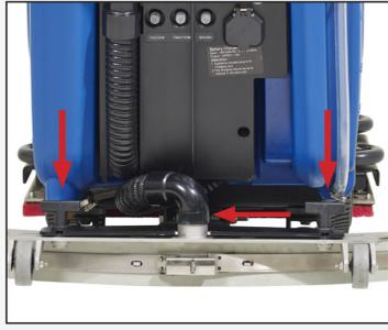
2. Install the squeegee using the thumb nuts. Attach squeegee hose.
