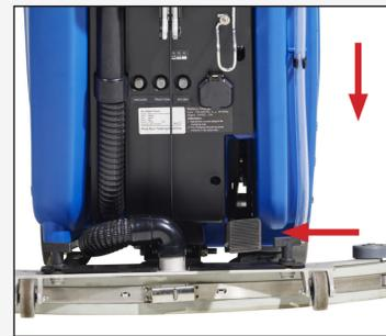
6. Lower the brush deck by pushing on the pedal to the right and lift it up.
