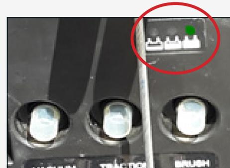
9. Daily: Charge the machine overnight and check the status using the battery status gauge.
