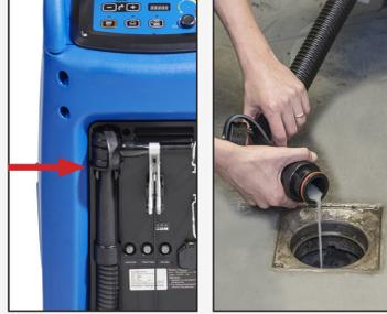
3. Daily: Empty the dirty water tank using the recovery water dump hose.
