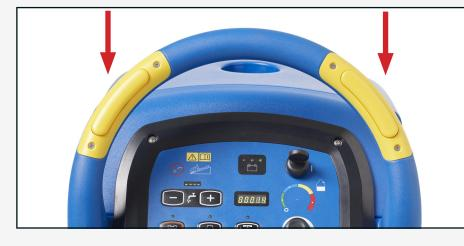
9. Press left, right or both yellow palm switches to move the machine forward.
