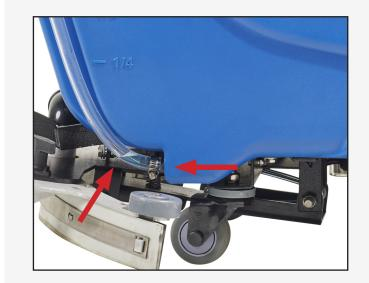
2. Daily: Empty the clean water tank using the solution tank drain hose and sight tube.
