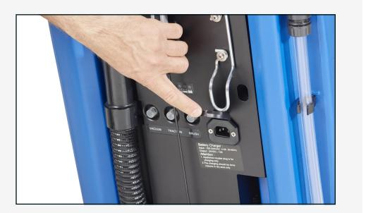
8. Daily: Charge the machine when not in use using the supplied AC cord and onboard charger receptacle.
