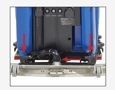
2. Install the squeegee using the thumb nuts. Attach squeegee hose.
