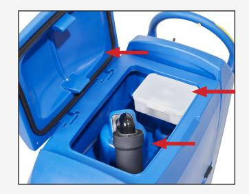
4. Daily: Inspect and rinse the ball float cage and the foam filter, debris catch cage and inspect and clean the gasket as required.
