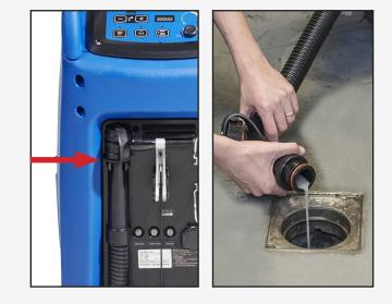
3. Daily: Empty the dirty water tank using the recovery water dump hose.
