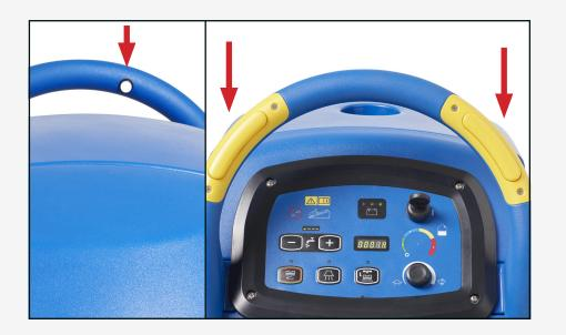
11. Pressing either yellow palm buttons and the white reverse button together will put the machine into reverse.
