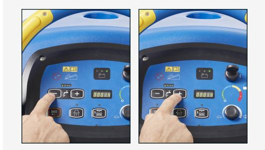
12. Press the + or – solution buttons to increase or decrease the water flow rate and to turn water off.
