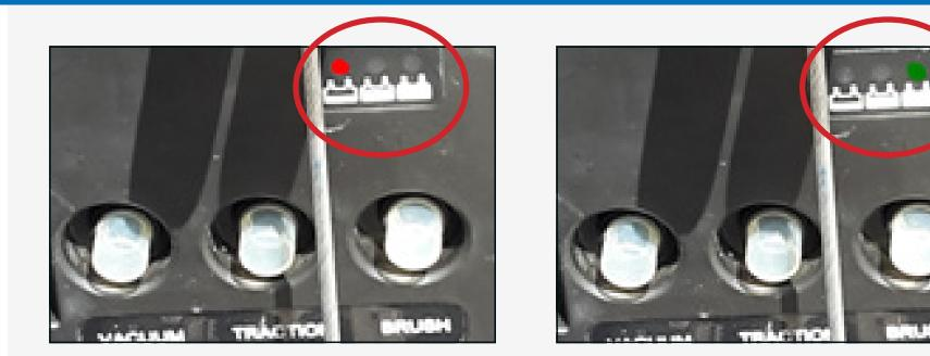
9. Daily: Charge the machine overnight and check the status using the battery status gauge.
