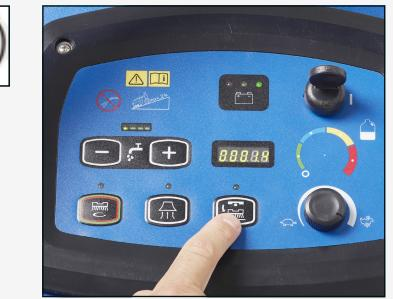
13. On disc machines, the brush/pad holder can be removed automatically.Raise the deck and press the click off brush button.
