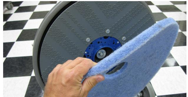
5. Check the pad holder for any damage or warpage.
