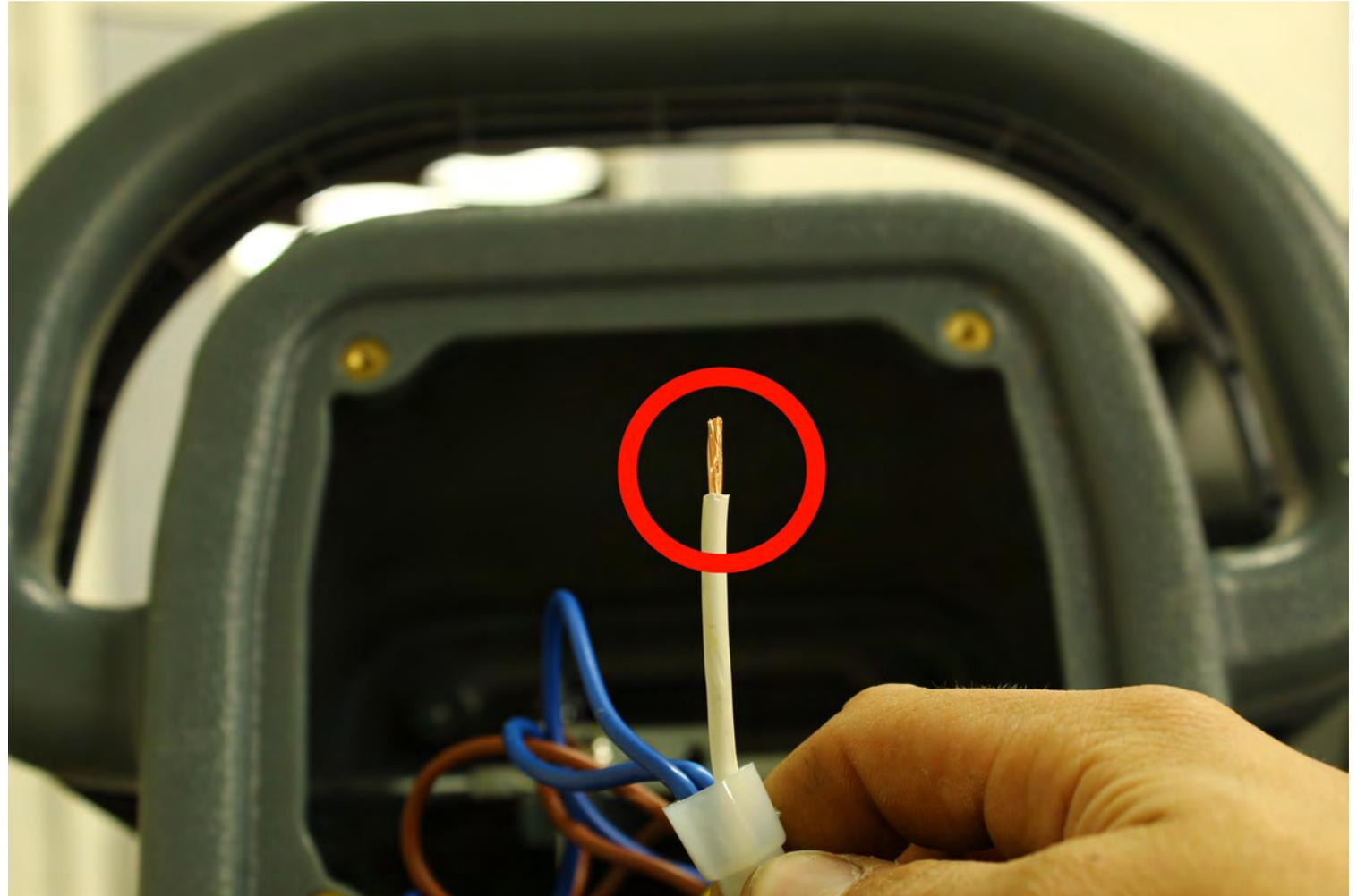
1. Install a new supplied connector on both the white and green wire
