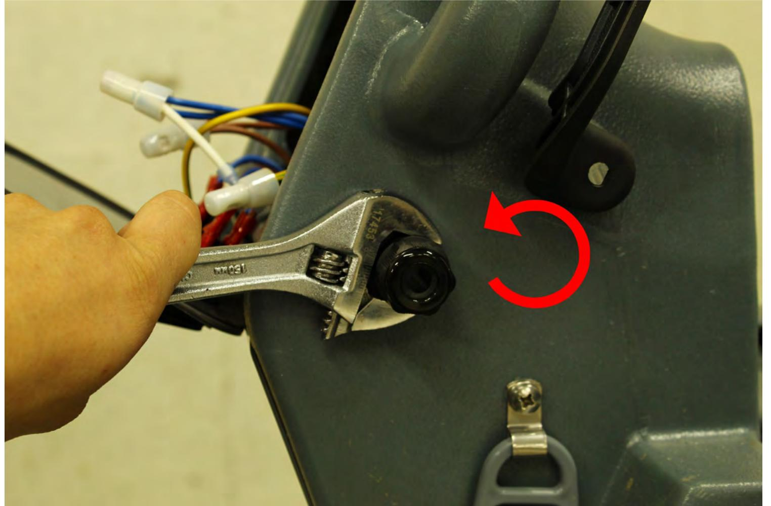
1. Insert the new strain relief and tighten
