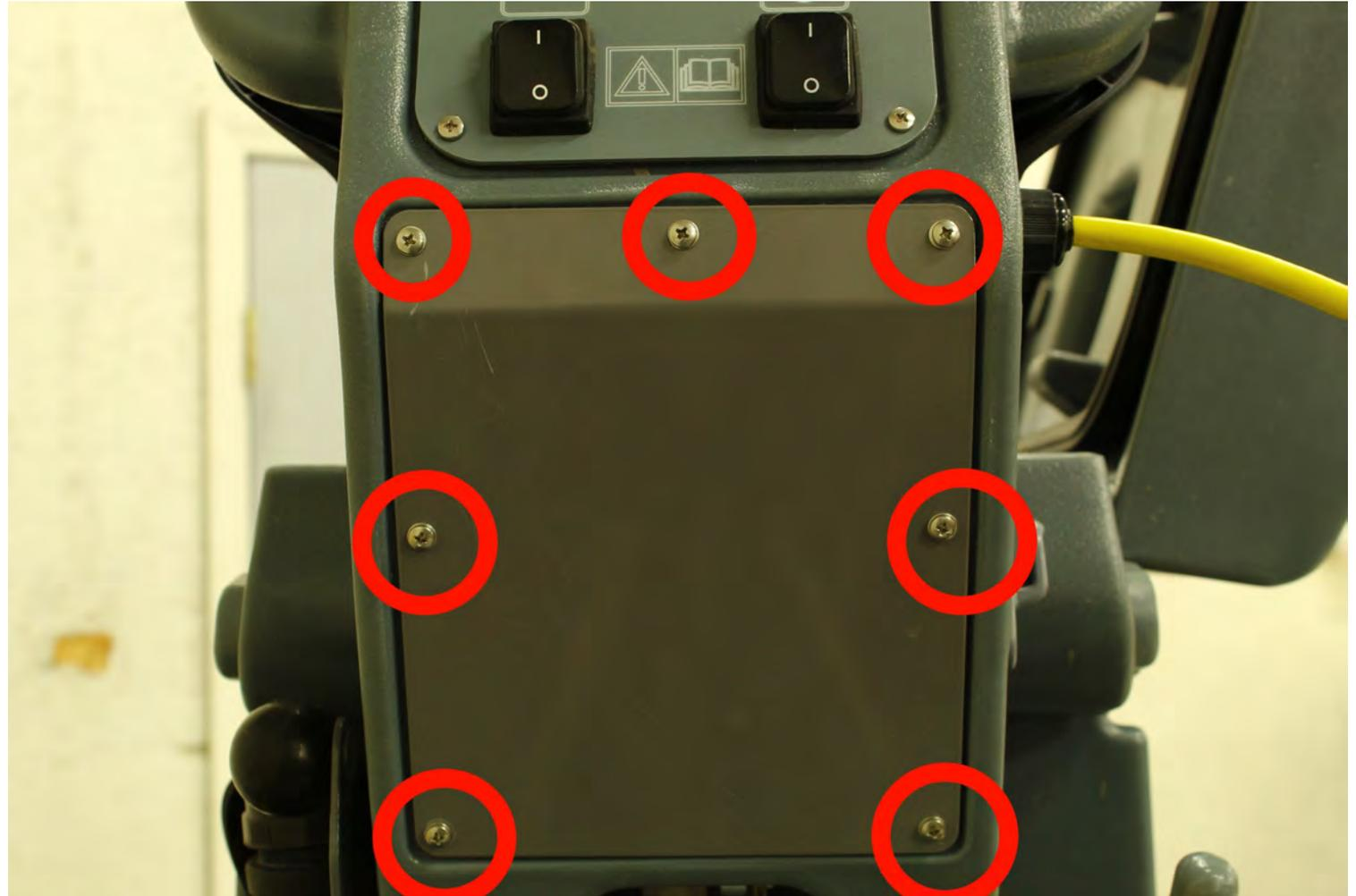
1. Install the 4 Philips head screws on the control panel.
