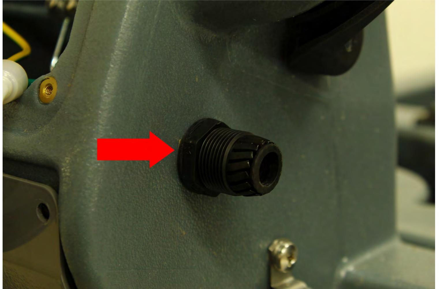
1. Remove the old strain relief, using a crescent wrench
