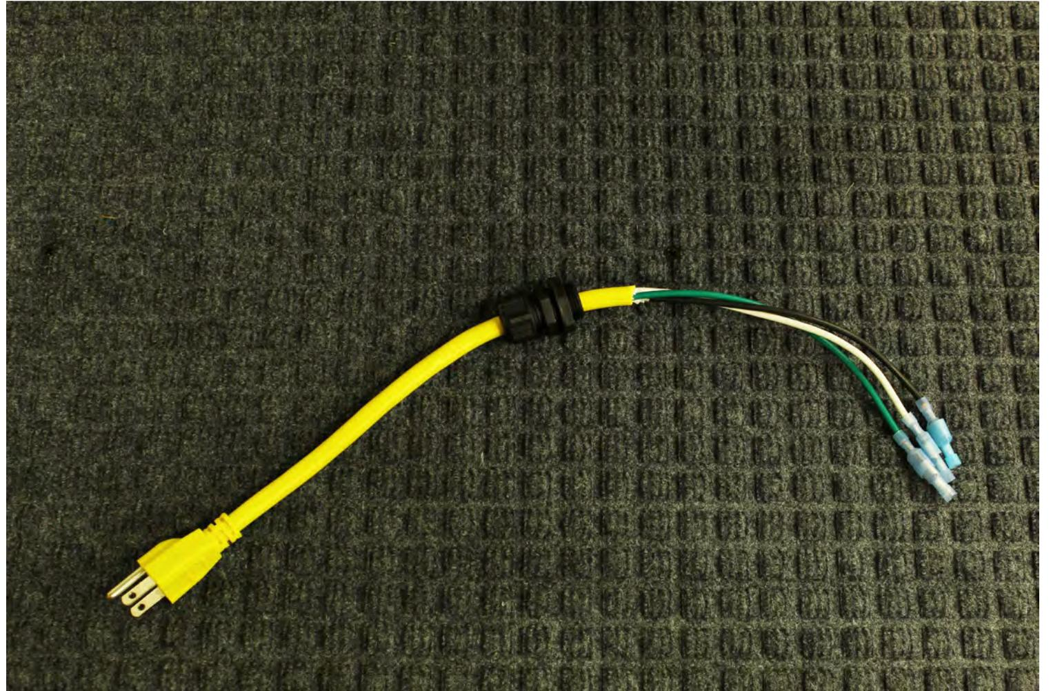
1. Connect the white and green wires from the Pigtail to the machines wire harness, as shown in the picture
