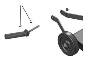
3. Insert the locking clamp handle/spade bolt assembly through the Cord Hook Clamp assembly (located on the handle) and the left and right handle braces ( D11481, D11482).
