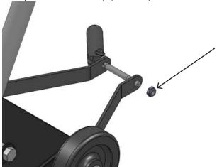
2. Slide out the locking clamp handle (D11497) assembly with spade bolt (C11536) and set it aside.
