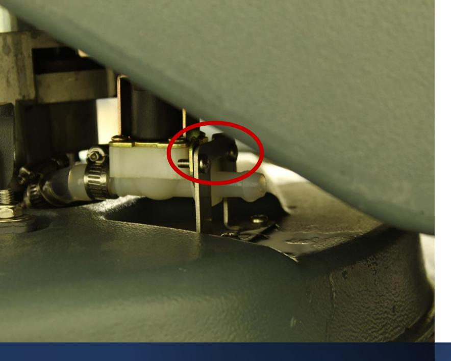
1. Screw in the 2 Philips head screws shown in the picture
