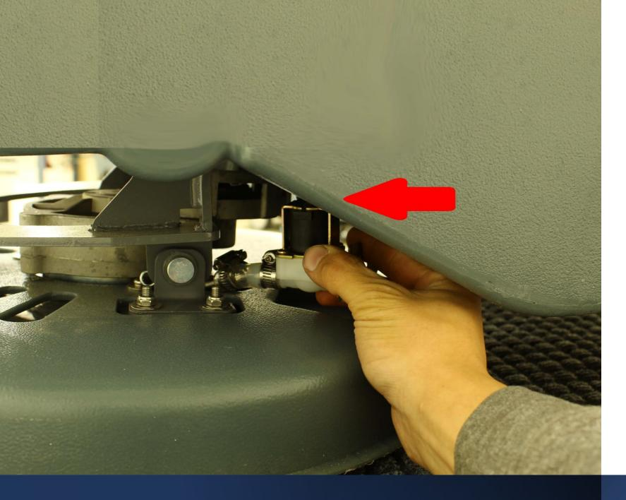
Insert the new solenoid back into the hose
