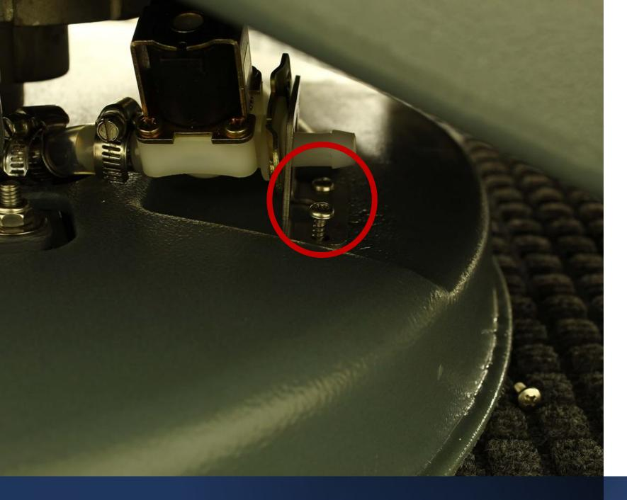
After removing the 2 Philips head screws, Remove the 2 Philips head screws holding the bracket to the deck
