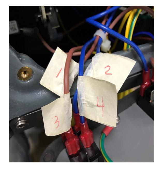
After labeling each wire, remove the wires carefully, remembering where each wire goes
