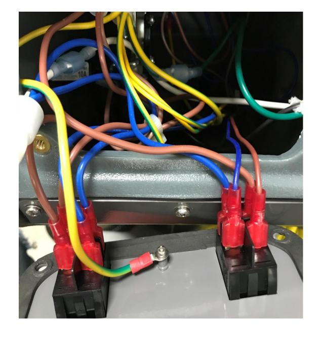
Add a piece of masking tape to each wire for future reference, label the corresponding wires in numerical order as shown in the picture
