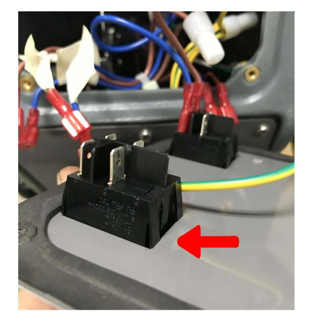
Pull the old switch out and replace with a new switch
