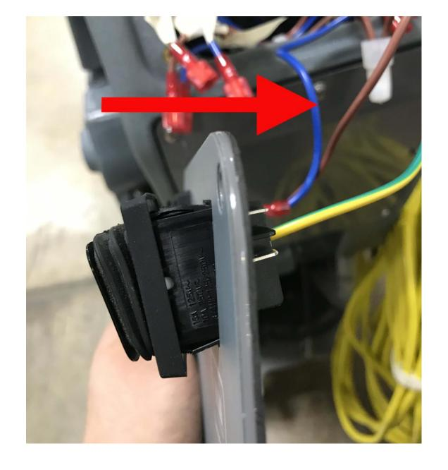
Plug the correct wires back into the terminals of the switch
