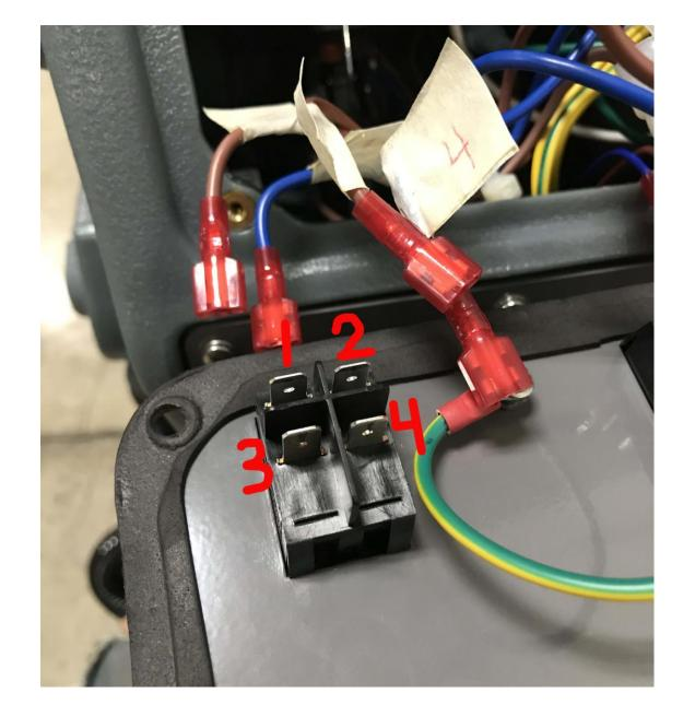
• Push the clip, on each side that holds the switch on the plate
