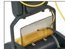
Stopper added to prevent lid touching drum during carpet encapsulation process
