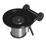
3. Use the four screws in the bag and mount the brush cover. Hand-tighten the screws first and then use a wrench to tighten them firmly. Use a CROSS pattern to tighten the bolts as shown below.
