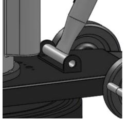
6. Place the handle in the down position to check the locking function. If too tight, unlock the handle and loosen the nut (C11558) slightly. If too loose, unlock the the handle and tighten the nut (C11558), as needed. You have assembled the cord hook clamp assembly properly when the locking handle locks firmly in the DOWN position and unlocks and slides easily in the UP position.
