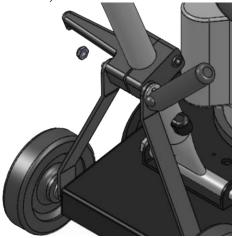
4. Put the locking clamp handle in the unlocked position (pointing up) and start tightening the nut C11558 on the threaded portion of the spade bolt (C11536).
