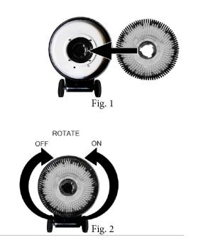
TO REMOVE PAD DRIVER: Tip the machine back so it rests on the
