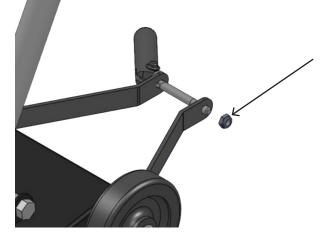
2. Slide out the locking clamp handle (D11497) assembly with spade bolt (C11536) and set it aside.
