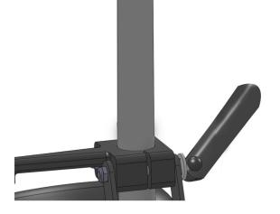
5. Check the cord hook clamp is sliding up and down freely on the handle stem with locking clamp handle in the unlocked position.
