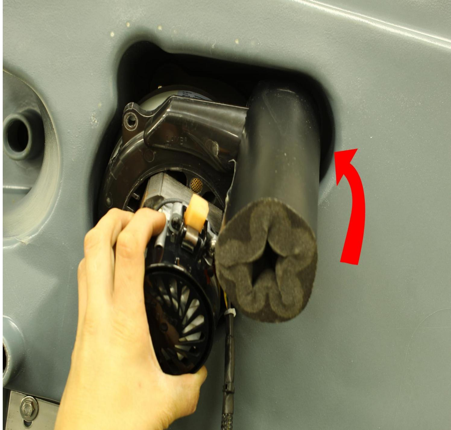
1. Tighten the 10mm nuts, BE CAREFULL NOT TO OVER TIGHTEN, OVER TIGHTENING WILL CAUSE THE VACUUM MOTOR TO CRUSH AND DAMAGE THE VACUUM MOTOR
