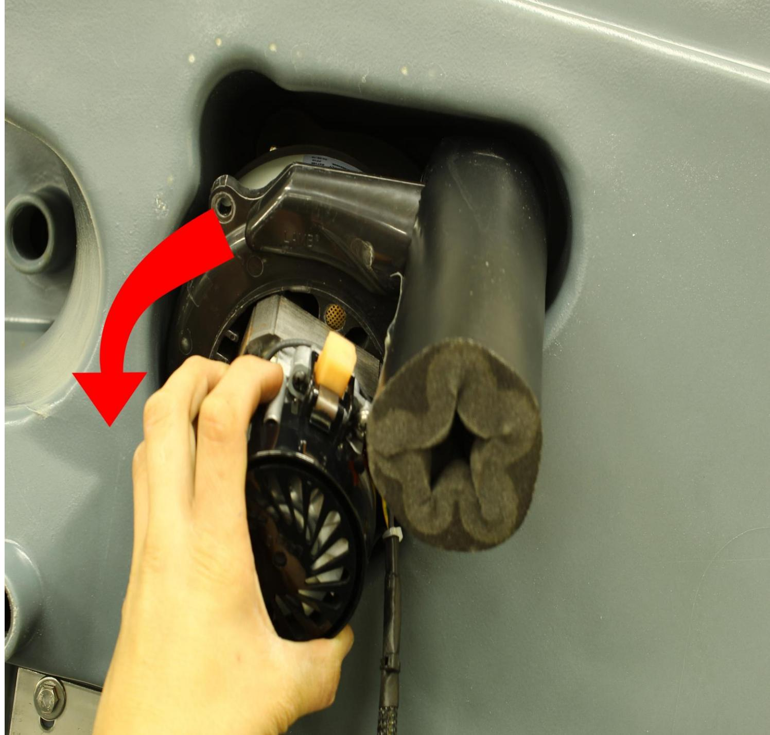
1. Remove the muffler from the motor carefully. Attach the muffler to the new vacuum motor.
