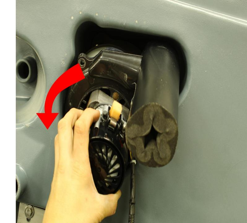
Remove the muffler from the motor carefully. Attach the muffler to the new vacuum motor.
