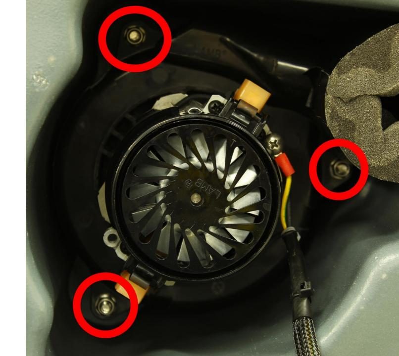
1. Remove the 3, 10mm nuts using an extension and a 10mm socket
