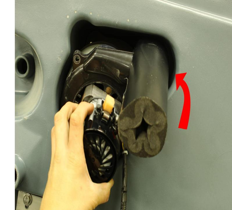
1. Tighten the 10mm nuts, BE CAREFULL NOT TO OVER TIGHTEN, OVER TIGHTENING WILL CAUSE THE VACUUM MOTOR TO CRUSH AND DAMAGE THE VACUUM MOTOR
