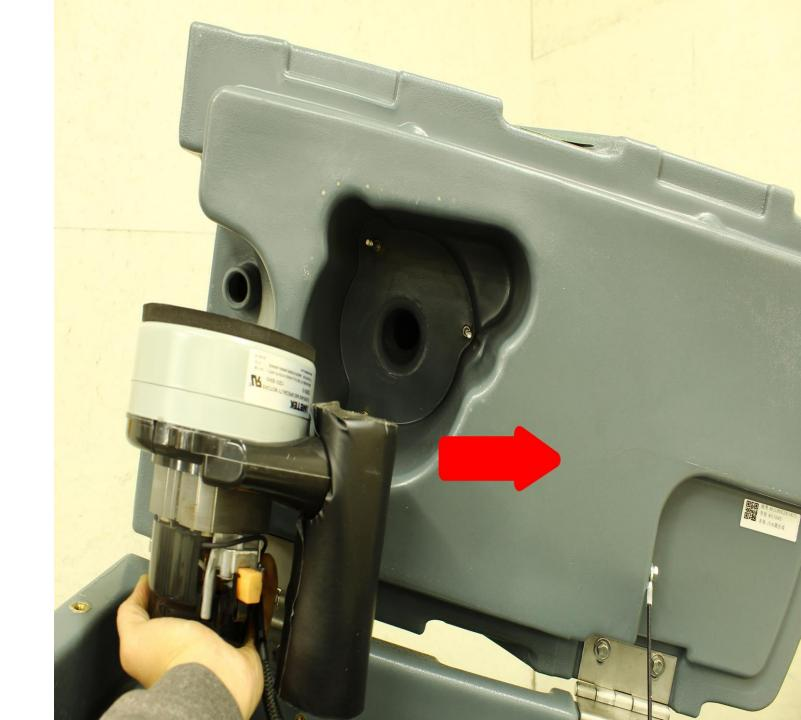
1. Carefully insert the vacuum motor back into mounting studs
