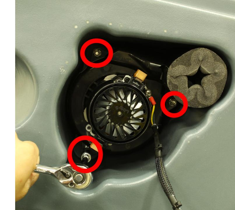
1. After removing the 10mm nuts, gently slide the vacuum motor out of the recovery tank mounting studs
