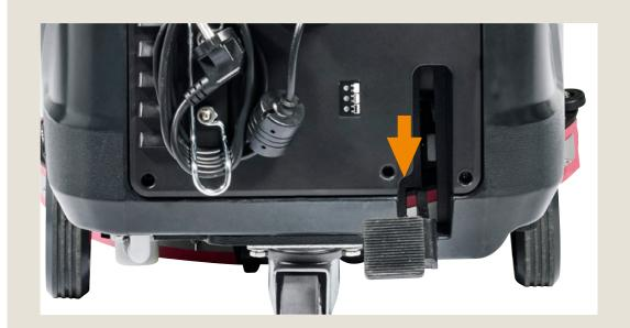
Lift the deck by pressing the pedal down and to the left. The squeegee is raised and lowered with the deck.
