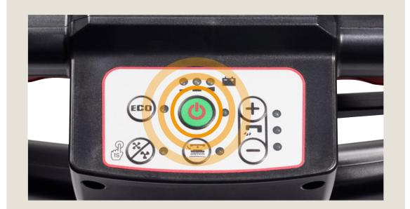
Turn on the machine and verify there is enough battery power to complete the work. Charge batteries if required.
