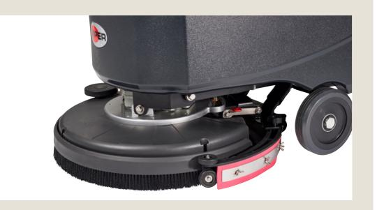
Place the brush or pad-holder under the center of the drive plate and lower the deck by pressing the foot pedal down and to the right.
