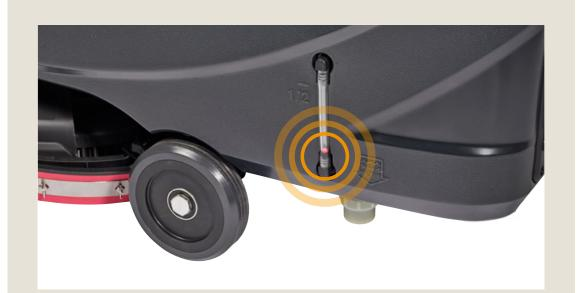
You can check the level of the solution anytime using the red ball on the left side of the machine.
