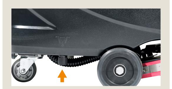
**Daily:** Empty the clean water tank using the solution tank drain knob under the machine.
