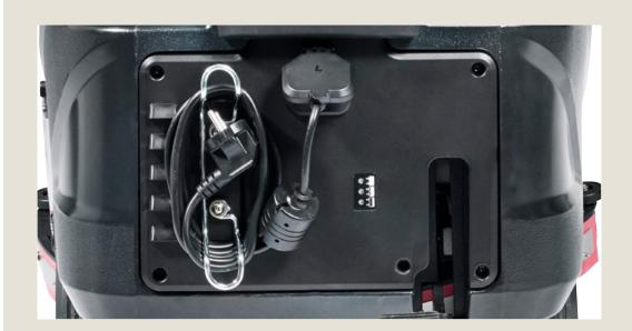
Charge the batteries whenever the machine is not in use. Connect the charger cable to the machine socket, then plug the cable into a grounded 3-prong electrical outlet. Red LED will be on during charging, and the Green LED will turn on when charging is complete.
