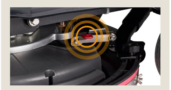
Lift the squeegee up by hand until it locks in the UP position, and turn off the vacuum, to perform double scrubbing. To return to normal working mode, use the red lever to release the squeegee, and turn the vacuum back on.
