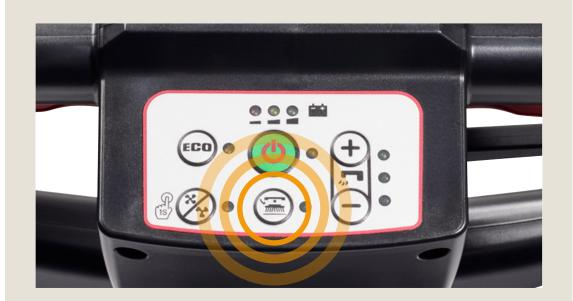
**Daily:** With the machine turned on and the deck lifted, press the click off button to release the brush/ pad holder then clean and inspect before next use.
