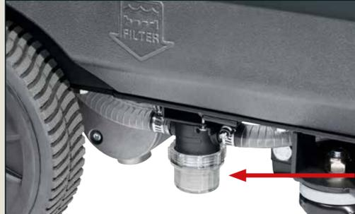
Weekly: Inspect the solution filter and clean if required.
