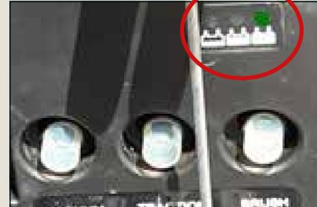
Daily: if the battery indicator shows red, put the machine on charge. Battery should be on charge if empty, not in use or if not being used for coming 8-10 hours.
