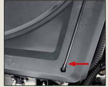
Check the level of water with the red ball on the left side of the machine.
