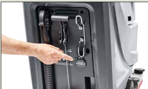
Daily: to charge the battery, use the supplied AC cord to the on board charger and connect it to the machine and wall socket.
