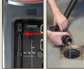
Daily: Empty the recovery tank using the recovery empty hose. Bend the soft part before removing the cap to control the flow.
