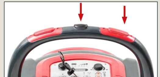
For wheel traction version: pressing either of the red safety switches and the black reverse button together will put the machine into reverse.
