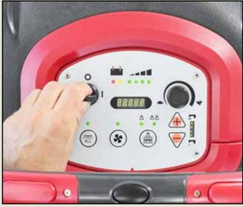
Turn on the key and verify there is enough battery power to complete the work. Charge batteries if required.
