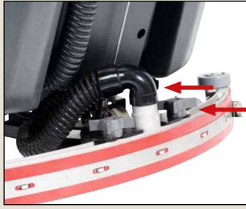
Install the squeegee using the thumb nuts. Attach squeegee hose.
