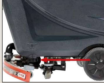
Daily: Empty the clean water tank using the solution tank drain knob under the machine.
