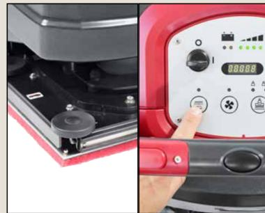
Disc version: place the brush/pad holder under the scrub deck then use the pedal to lower the deck over the brush. Press the OneTouch™ scrub button to enable scrubbing. The vacuum will start. Push on one of the two switches ½ second to install the brush.
