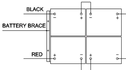
5. Apply a coat or protective spray on the cable connections to prevent battery corrosion.
